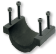
Spacer Spacer for Ring Base & Top and Twist Mounts. Raises height of optical axis from 30 to 39 mm Art. No. 12227 *
