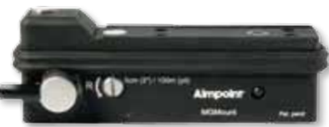
MGMount for MPS3 Contains a 3-step ballistic compensation for 200, 800 and 1200 meters (220, 875, 1310 yards) distances. The mount is also used to zero the MPS3 sight. Export license/End-user certificate is required for this product. Art. No. 11925 * NSN No. 1240-01-551-6720
